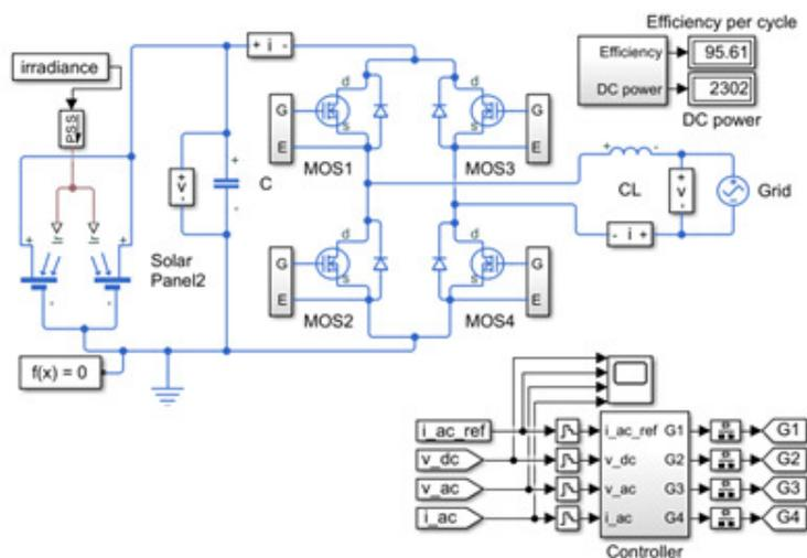
**Fig. 3** implementation solar power converter by simulink matlab
