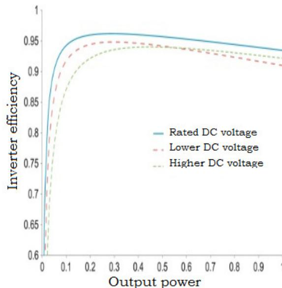
**Fig. 1** Typical inverter efficiency curve as a function of DC input voltage
