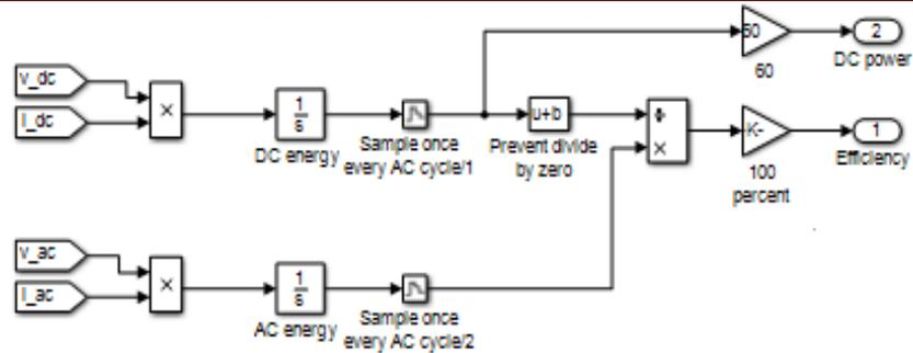
Fig.4 Calculation efficiency end DC power of solar power converter
